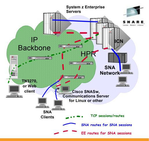
EE allows enablement of IP applications and convergence on a single network transport while preserving SNA application and endpoint investment.
