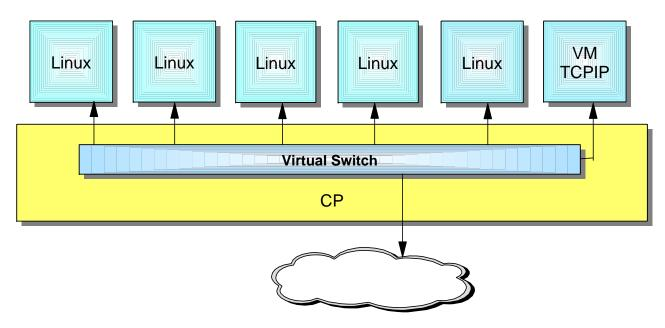
New Virtual Switches allow virtual QDIO connections to physical LAN segments without requiring a router
