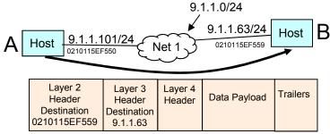
• For Host A to send data to Host B, 9.1.1.63, on the subnet that it is attached to (Direct Route) it uses ARP to learn the MAC address, 0210115EF559. The Layer 2 header is created with the destination 0210115EF559.
