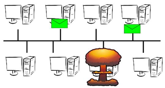
The interdependence between systems can be decoupled through the use of a common messaging system, providing a scalable environment which is more tolerant of individual system outage.
