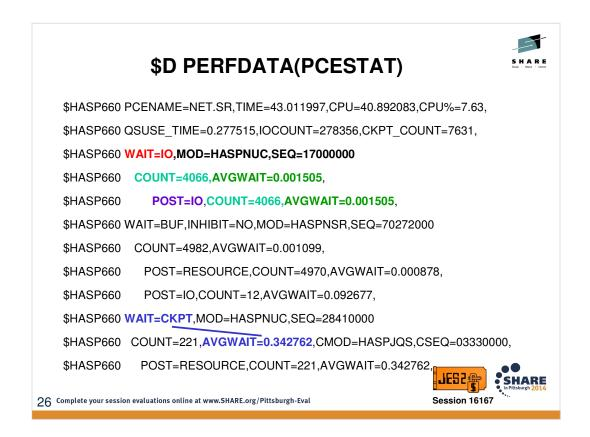
This section starts with the CPU statistics (CPUSTAT), and then follows with a breakdown of activity of that PCE type. Specifically, it will breakdown the PCE \$WAITs and \$POSTs by type and count. The AVGWAIT for WAIT=CKPT help give insight into CKPT access time. All wait times include queue time for the PCE type – the time it is on the ready queue awaiting dispatch.
