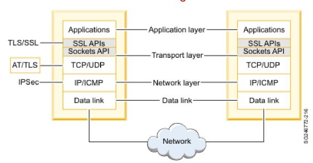
AT-TLS is activated by specifying the TTLS option in the TCPCONFIG statement block in the TCP/IP profile data
