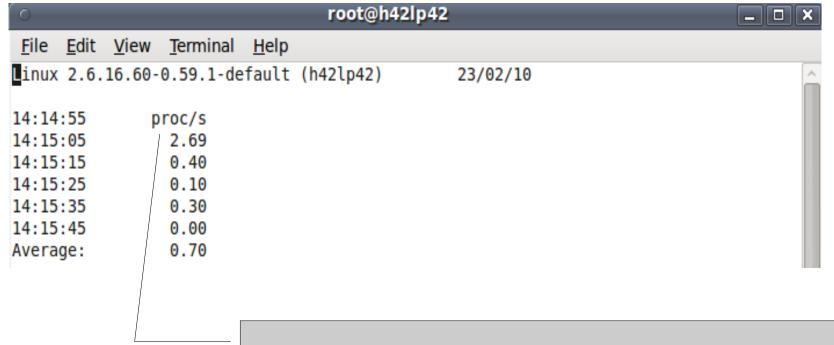
Processes created per second usually small except during startup. If constantly at a high rate your application likely has an issue. Be aware – the numbers scale with your system size and setup.
