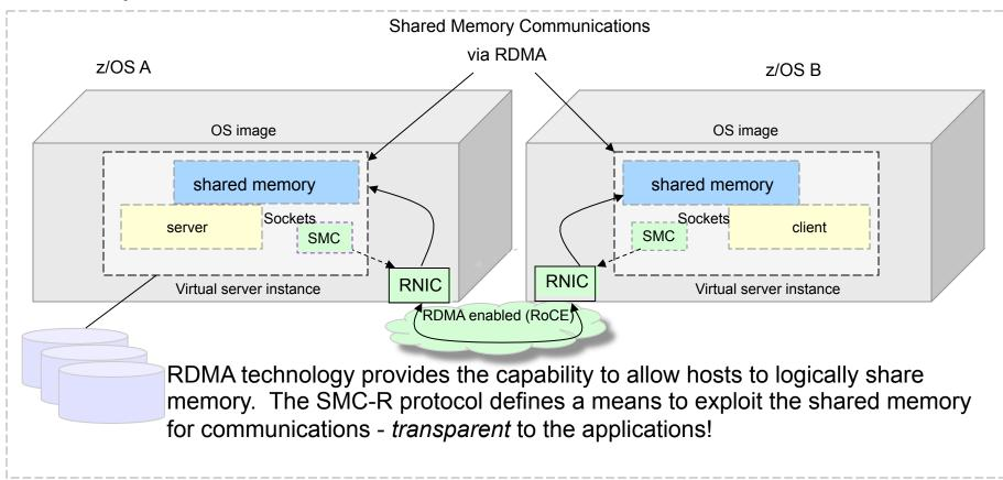
This solution is referred to as *SMC-R* (Shared Memory Communications over RDMA). SMC-R is an *open* sockets over RDMA protocol that provides transparent exploitation of RDMA (for TCP based applications) while preserving key functions and qualities of service from the TCP/IP ecosystem that enterprise level servers/network depend on!
