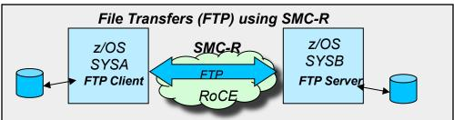
Up to 50% CPU savings for FTP binary file transfers across z/OS systems when using SMC-R vs standard TCP/IP \*\*
