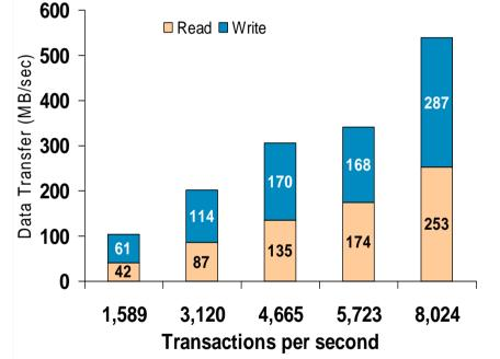
System z easily surpassed benchmark goal, and demonstrates near linear scalability Reads and writes are well-balanced and scale linearly, demonstrating no constraints on I/O
