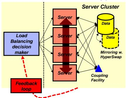
In order for the load balancing decision maker to meet those objectives, it must be capable of obtaining feedback dynamically, such as server instance availability, capacity, performance, and overall health.
