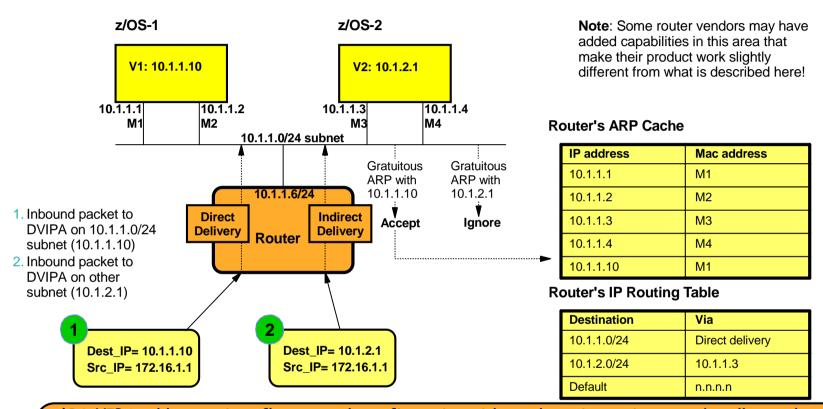
z/OS VIPA addresses in a flat network configuration without dynamic routing must be allocated out of the same subnet as the directly attached network that all members of the Sysplex are attached to in this example, the 10.1.1.0/24 subnet.
