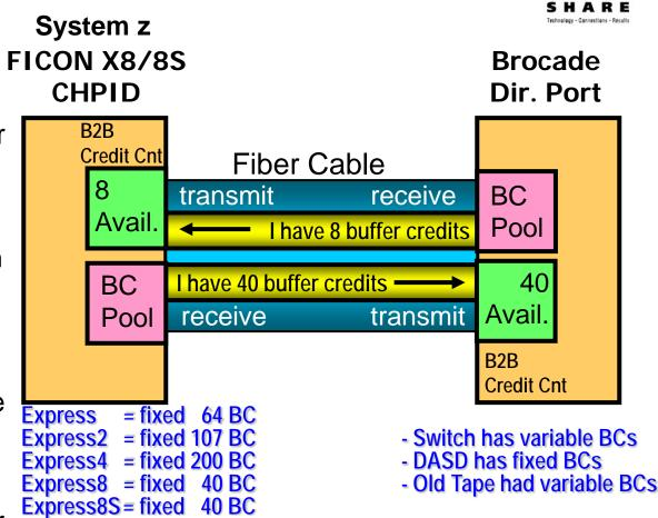
Each receiver on the fiber cable can state a different value!
