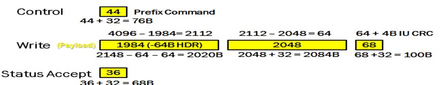
4K will not fit into 2 BCs because of headers for FC as well as SB3 protocol that is used and the 64 byte FICON header that is placed into the payload field of the 1<sup>st</sup> frame of every FICON exchange.
