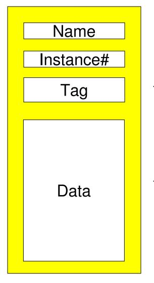
8 byte user note name8 byte XCF instance number16 bytes of user metadata
