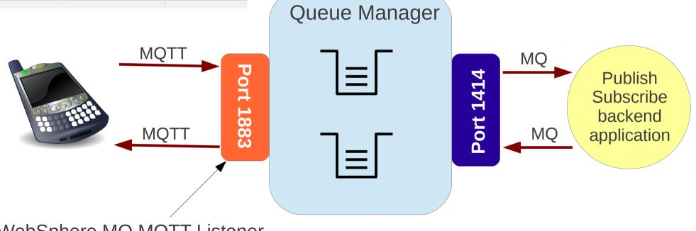
WebSphere MQ MQTT Listener IANA registered ports: 1883, 8883 for MQTT over SSH
