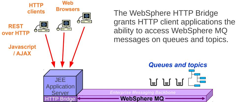
The HTTP Bridge comprises of a JEE Web application (servlet), which is to be installed into a JEE Application server in order to be used.
