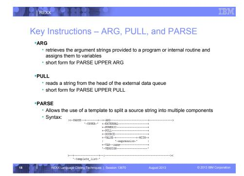
PARSE EXTERNAL - used in z/OS to read from the terminal if running interactively, or from DD SYSTSIN if running in batch
