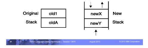
•NEWSTACK command creates a private data stack that is completely isolated from the original data stack
