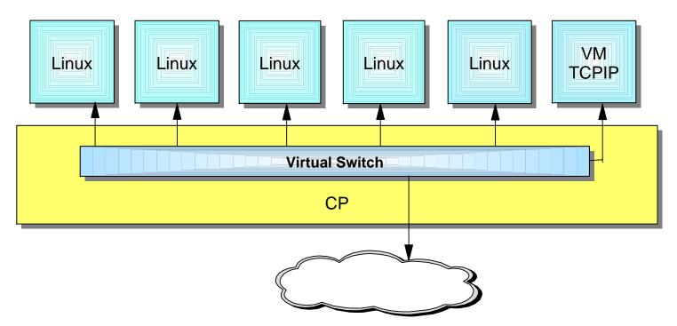
New Virtual Switches allow virtual QDIO connections to physical LAN segments without requiring a router
