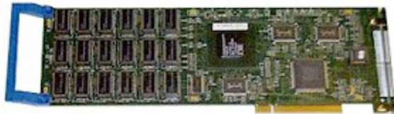
A complete System/390 processor on a single PCI card.
