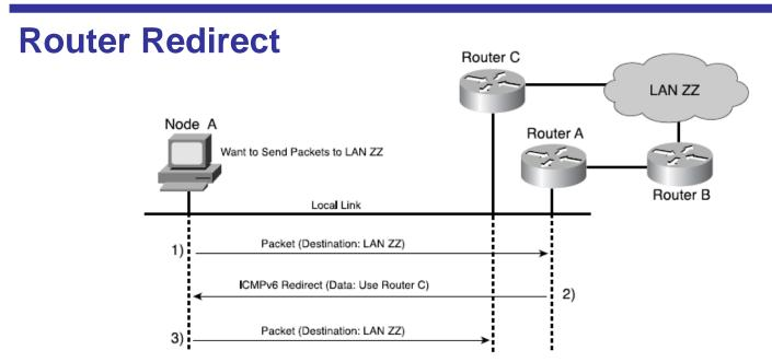
1. A router informs an originating host of the IP address of a router available on the local link that is "closer" to the destination.
