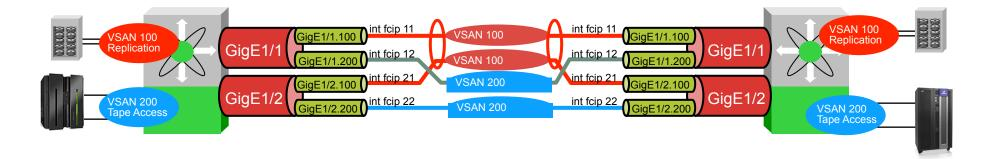
Using GE Sub-Interfaces, Multiple FCIP Tunnels and Port Channeling to Enable High b/w FCIP
