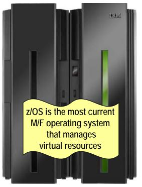
z/OS can run in up to 60 partitions on a M/F or it can be intermixed with other operating systems running in other LPARs Z Operating System (z/OS)
