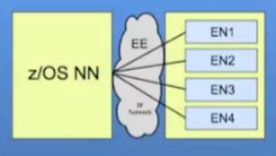
Improves throughput for EE connections to virtualized servers or CPU-constrained endpoints
