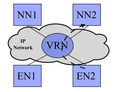
Example: Since EN2 and NN2 both define the VRN, a dynamic connection can be activated between them over the VRN without predefining a static EN2-to-NN2 connection
