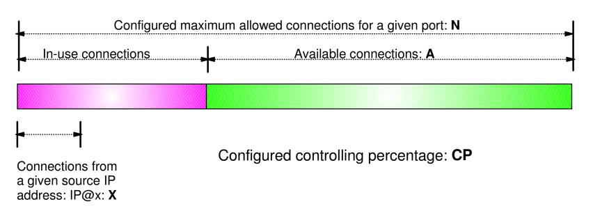
If a new connection request is received and A=0, the request is rejected.
