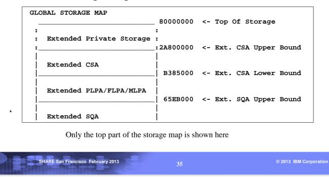
VERBX VSMDATA with a parameter of NOASIDS provides a global storage map that shows the boundaries of different area of storage for every address space. This will allow you to figure out whether the address at hand is in private or common. To see the details of the private storage of an address space see next page.
