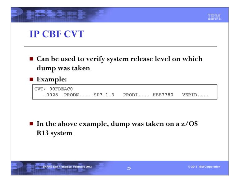
This is important because you should use the same level of IPCS as the z/OS release of the system on which the dump was taken. IPCS will put out a message if you use a level of IPCS that is different than the level of the z/OS system on which the dump was taken.
