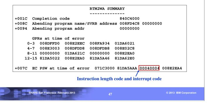
If the TCB is going through recovery processing for the error in the completion code, you will find a RTM2WA (RTM2 Work Area) after the TCB. The above shows the RTM2WA Summary which contains the PSW at time of error and the registers, as well as the instruction length code, interrupt code, and the translation exception address (not applicable in this case since the interrupt code represents a protection exception).
