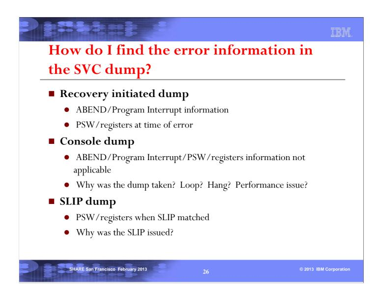
There is always a set of PSW/register information crucial for debugging a recovery-initiated dump or SLIP dump.
