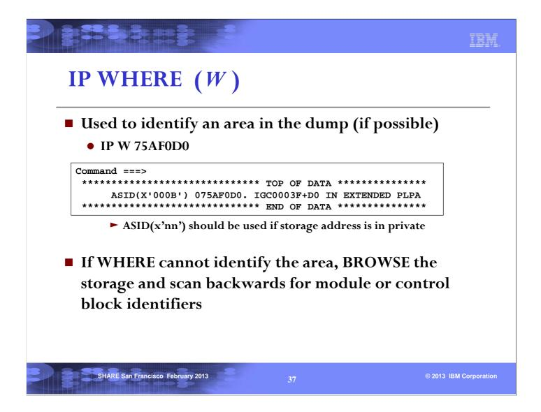
For an address that may point to a module or a common control block, the IPCS WHERE subcommand can be used. Note that the ASID parameter should be used if the address is in private storage.
