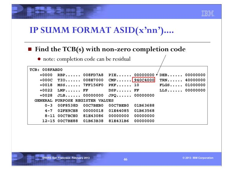
Once you found a TCB with non-zero completion code, you can issue a FIND of 'TCB: 00xxxxx' from the top of the output to find the TCB. The error under this TCB may be the one causing the dump to be taken. Or it can be a residual completion code.
