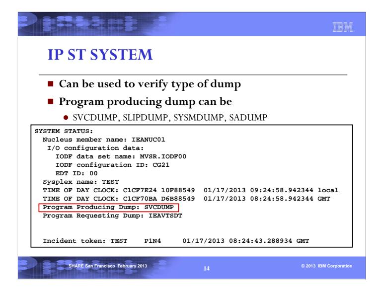
The time provided is the time that global data capture completed. This is an example of an SVC dump.
