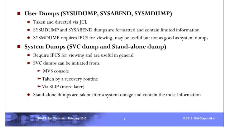
The basic problem documentation is a dump. Dumps give a picture of the failing program and the system at the time of the problem. We do not usually find user dumps very useful in debugging z/OS problems, so make sure you collect an SVC dump for a problem.
