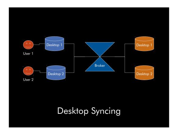
This is when the users sync the desktop when the are done using it. This is used when the user still has a thick client but is not attached to the corporate data center. This is important for mobile users.
