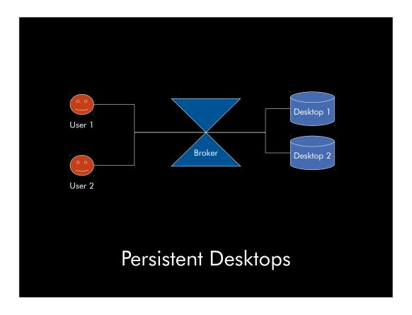
One way to build a VDI is with persistent desktops. The user request the exact same desktop every time, though it is there person desktop. Generally this is a full replace for the standard no VDI based desktop.
