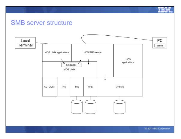
The SMB server runs as an authorized started task in its own address space. It accesses z/OS UNIX files on behalf of PC users. It can also access MVS data sets on behalf of PC users.
