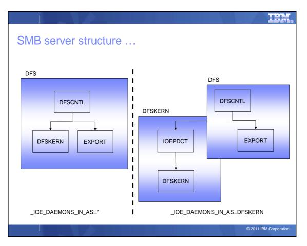
The DFSKERN process (which is the main server process) can run in the DFS address space (the default - shown on the left) or in its own address space (shown on the right). IBM recommends that you run DFSKERN in its own address space. This is accomplished by specifying \_IOE\_DAEMONS\_IN\_AS=DFSKERN in the /opt/dfslocal/home/dfscntl/envar environment variable. The DFSKERN JCL must also be available.
