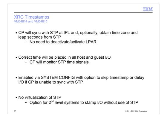
CP will sync with correct time from STP at IPL STP is not virtualized to 2<sup>nd</sup> level guests CP will track time changes (drift) – will be put in timestamps for I/O
