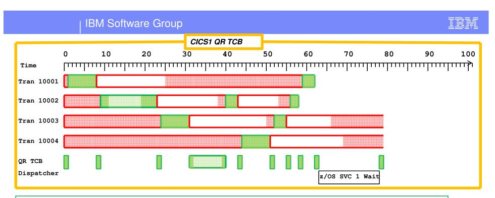
•During that time, notice 2 transactions became dispatchable. Typically the TCB would wake up out of its wait immediately when a transaction becomes dispatchable. The reason that didn't happen is probably because the processor was not available.
