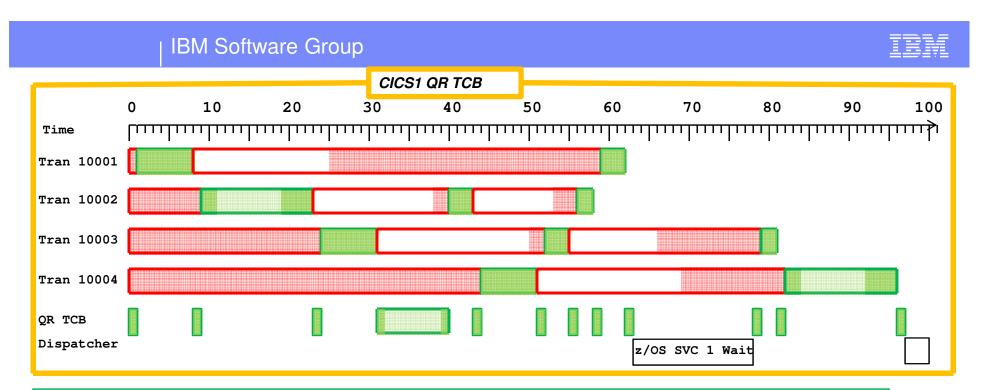
•Here the last 2 tasks finish up. Transaction 10004 lost control of the TCB for some reason during its last dispatch.
