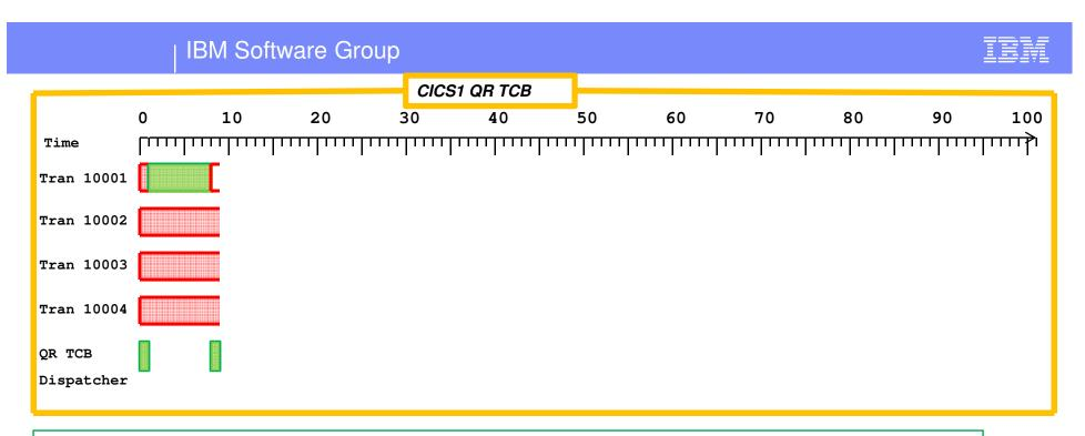
•Tran 10001 received control. It held control of the TCB for 7 units of wallclock time and then it suspended giving control back to the CICS dispatcher.
