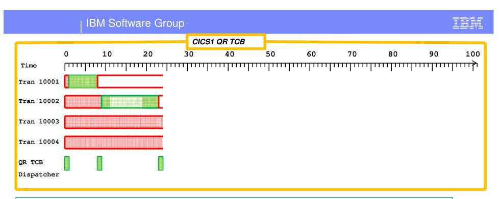
•Transaction 10002 had control of the TCB for 13 units of time. But this time it used only 7 units of CPU. So while transaction 10002 was in control of the QR TCB, the QR TCB stopped executing instructions for some reason. Maybe z/OS took control away to let higher priority work use the processor.
