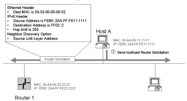
To forward packets to off-link destinations, Host A must discover the presence of Router 1.
