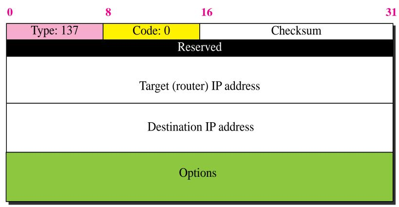
An option is added to let the host know the target router's physical address.
