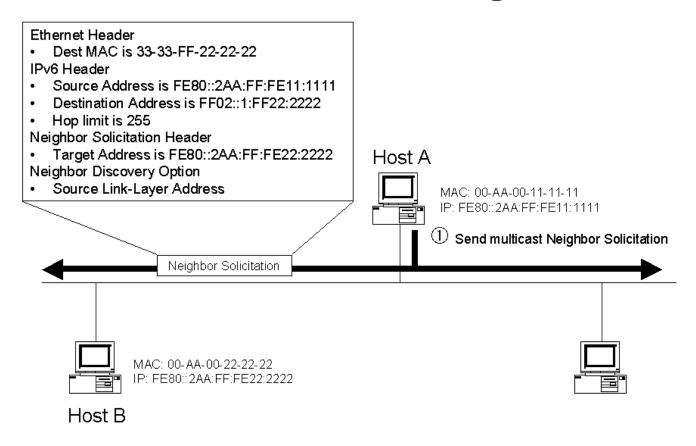
To send a packet to Host B, Host A must use address resolution to resolve Host B's link-layer address.
