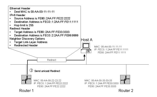
To inform Host A that subsequent packets to the destination of FEC0::2:2AA:EE:FE99:9999 should be sent to Router 2, Router 1 sends a Redirect message to Host A.
