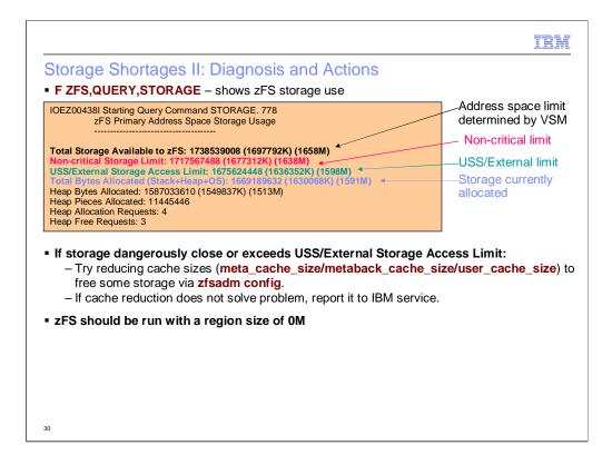
If zFS is low on storage, one possible method of freeing some memory is to reduce cache sizes via the zfsadm config command. The query storage command will also show a per-component breakdown (not shown here) which can be used to determine which cache is the best to reduce in size. Generally speaking, when increasing caches due to performance tuning, be careful not to make them too large for zFS primary storage; you want to prevent a storage shortage rather than correct one.
