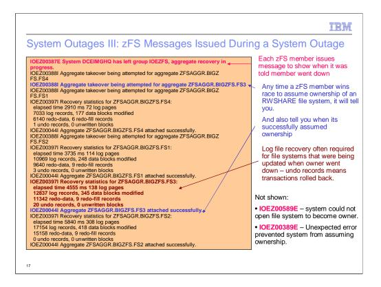
Shown on this slide are the messages specifically related to down-system recovery processing. While other errors could occur during recovery processing (such as an unexpected disk IO error for example), these messages show the general flow of ownership assumption and whether the system successfully assumed ownership or not.
