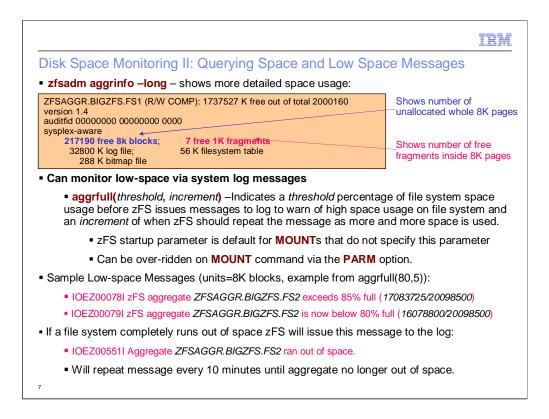
The zfsadm aggrinfo –long is the most informative command to use to determine how much free space there is in a zFS file system. It shows the number of whole 8K pages that are unallocated on the disk. As long as this number is not 0 any object can be grown in size, as soon as its 0 then any larger object cannot be grown in size. The command also shows the amount of space used for file system control objects.
