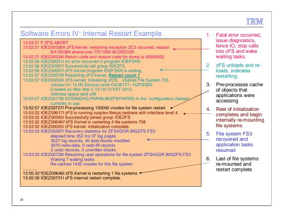
Its important to note that the application users of file system ZFSAGGR.BIGZFS.FS3 are running again as soon as message IOEZ00728I is issued. This restart was from a high stress workload against a zFS with very large caches and applications that were accessing a very large number of objects.
