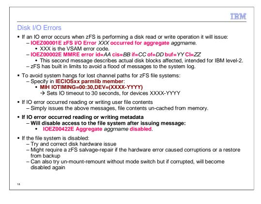
zFS will always issue messages IOEZ00001E and IOEZ00002E for disk IO errors that occur to a file system; zFS has limits to keep the number of messages shown per-file system to a reasonable amount. IOEZ00002E is intended for IBM service personnel.
