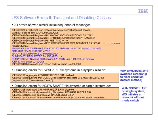
Transient errors only issue the PSW/register dump messages and show the return and reason code for the x2C3 dump zFS issues.
