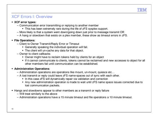
The one difference between a hang/slowdown and a lost transmit or reply packet is that there is still a task doing that work on the member that took too long processing the message; zFS handles those cases and will ensure that zFS systems stay consistent with each other and prevent improper sysplex access to file system objects and will repair zFS file system name-spaces.
