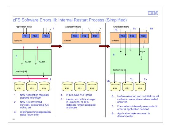
zFS internal restart is designed to handle fatal errors; hence, errors that significantly affect zFS operation or errors in error recovery (leaving something in an inconsistent state) and is a method to avoid a system-IPL.
