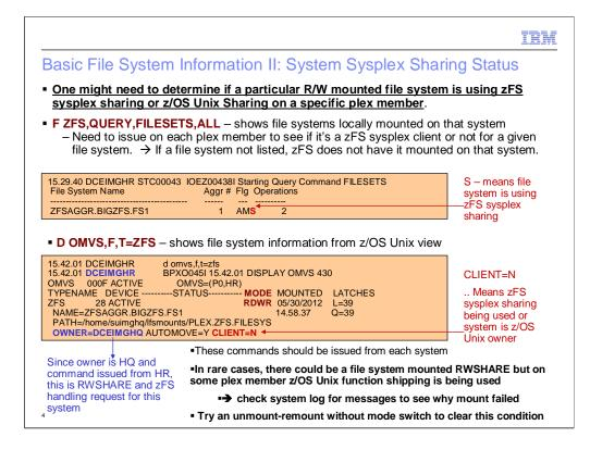
At mount time a R/W mounted file system will be mounted as RWSHARE or NORWSHARE in a sysplex. If the file system is mounted NORWSHARE then z/OS Unix sharing is used and z/OS Unix function ships requests from non-owner systems to owner systems. In this case the CLIENT=Y will be specified for each member that is not the owner, and CLIENT=N will be displayed on the system that is the owner of the file system.
