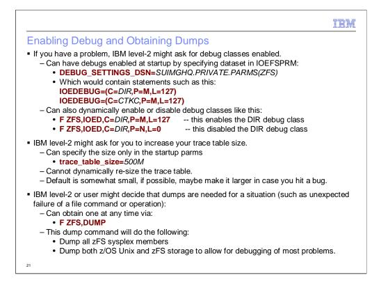
A customer would not generally enable zFS debug classes unless requested by IBM service. IBM service would provide instructions similar to those listed on this slide for ensuring proper documentation is obtained and request a dump (if one is not being auto-generated by zFS) via the F ZFS,DUMP command. One thing to keep in mind is that the zFS trace table currently cannot be dynamically re-sized (this should be fixed in a future release).
