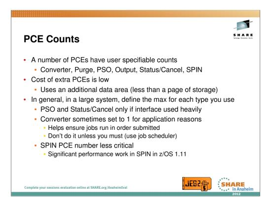
The number of certain PCEs can be specified via an initialization option. The PCEDEF initialization statement control the number JES2 defines. It can only be specified at initialization (no commands to adjust the number). In general, a large system should set these values to the maximum. There is little cost (performance or resources) but lots of benefits. However, there are some PCEs that you may not want to increase the number of:
