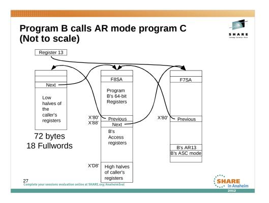
Program B can then call an AR mode program that requires a 216-byte save area. AR mode program C does not know or care that the high halves of program A's registers are stored at offset 216 of program B's save area.
