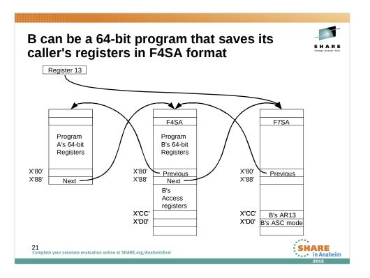
Here, program B is a 64-bit program that does not use Access Registers. It requires a 144-byte save area to save program A's registers in F4SA format. Program B will be calling program C, which does use the Access Registers. Program B knows that it must provide a 216-byte save area for C to save B's registers.
