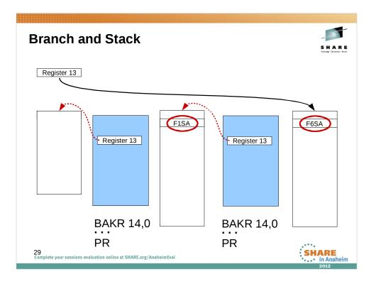
There is another way to save the caller's registers that does not use the save area that is passed in register 13. When a program issues a BAKR 14,0 instruction, the registers are saved on the Linkage Stack for the current task. The Return PSW in the stack entry contains the current PSW modified with the instruction address in Register 14.
