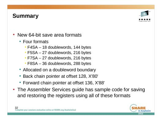
144-byte, 216-byte and 288-byte save areas are all allocated on a doubleword boundary.
