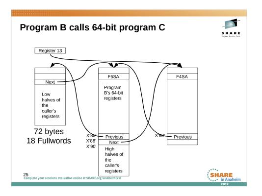
When program B calls another 64-bit program, the first 144 bytes of program B's save area can be used to store the registers in F4SA format. As with F4SA, a 31-bit program that is called by B will save the 32-bit registers with no ill effects.
