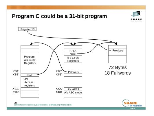
B can also call a 31-bit program. The 31-bit program will use the first 72 bytes of the 216-byte save are that was allocated by B. No harm is done by this. The 31-bit program saves its caller's registers in the usual way and the save areas are chained according to the rules for standard save areas. Offset 4 of the new save area has the address of the caller's save area. Offset 8 of the caller's save area is updated with the address of the new save area. The result is as is shown here.
