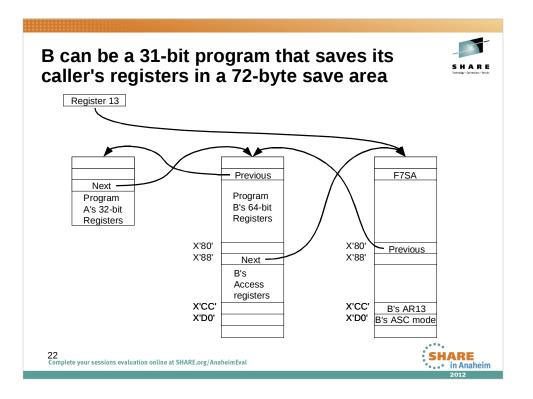
In this illustration, program B is a 31-bit program. It uses a 72-byte save area to save program A's registers in standard format. Program B will be calling program C, which requires a 216-byte save area for C to save B's registers. This might be unusual, but it is consistent with the rules for save areas.
