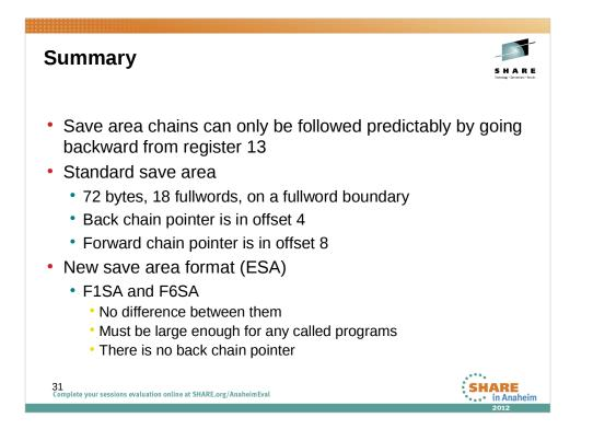
The backward chain is a necessary part of the save area. Every program must be able to find the save area where it saved its caller's registers. The forward chain is not required and there are two possible locations for it. As a result, the only predictable way to follow a calling chain is going backward.
