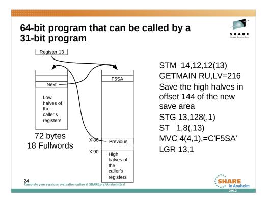
When a 64-bit program is not able to control its callers, it can not require that a 144-byte save area be passed to it. In that case, the low halves of the registers are saved in the caller's save area. A 216 byte save area is allocated and the high halves are stored at offset 144 of the new save area.
