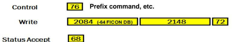
4K will not fit into 2 BCs because of headers for FC as well as SB3 protocol that is used and the 64 byte FICON header that is placed into the payload field of the 1<sup>st</sup> frame of every FICON exchange.
