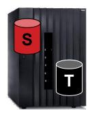
PiT copy technology on the disk subsystem When a FlashCopy is issued the copy is available immediately A bitmap tracks the relationship between source and target tracks
