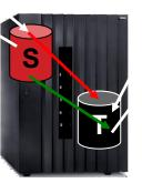
Writes to the source may cause a copy on write if the track has not been copied to the target
