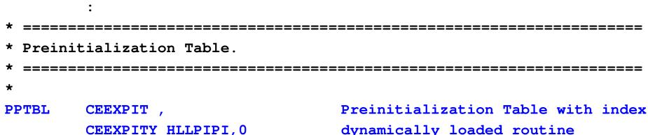
CEEXPITY HLLPIPI,0 CEEXPITY ,HLLEXTRN CEEXPITY , CEEXPITS , dynamically loaded routine statically-bound routine empty Table slot Endof PreInit table
