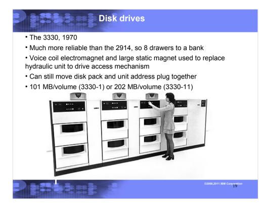
The IBM 3330 Data Storage (seen here in a design model) was a highperformance, high-capacity direct access storage subsystem for use with all IBM System/370 models as well as the IBM System/360 Model 195. Each 3330 subsystem could have from two to 16 drives, giving users up to 1.6 billion bytes of online storage. Developed and manufactured at IBM's facilities in San Jose, Calif., the 3330 was announced in 1970 and withdrawn from marketing 13 years later.
