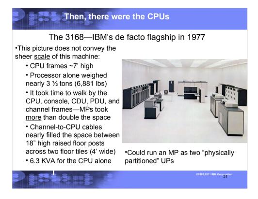
The 3168 is shown with its Power and Cooling Distribution Units (PDU and CDU) behind it to the left and its console ahead of it; a 3803 control unit & 3420 tape drives to the far left; a 3830 control unit & 3330 disk drives on the far right; a 327x terminal, 3505 reader & 3525 punch in the left foreground; and 3211 printers in the right foreground. I can't identify the box in the far right rear; it might be a 2701 or 2703 communications controller.
