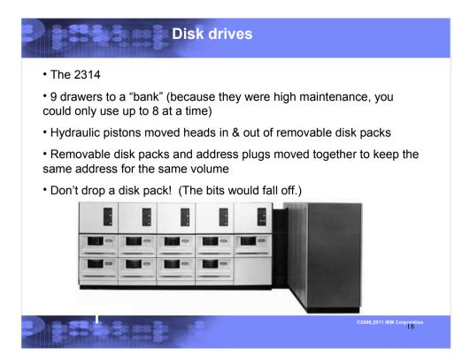
Introduced in 1965, the IBM 2314 Direct Access Storage Facility provided eight independently operating disk drives and a spare along with a control unit in one facility. Users of large-scale computer systems could attach enough 2314s to provide nearly 10 billion bytes of data storage.
