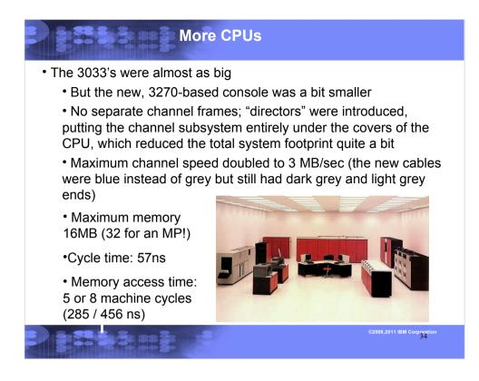
3033 shown with PDU and CDU to the back left and L-shaped 3270-based console in front. 3800 printer on the left has the optional Burster/Trimmer/Stacker feature; it's next to a 3505 card reader and 3525 punch. The box to the right rear might be a 3851 Mass Storage Subsystem (MSS). 3330s to the far right may have been MSS staging drives; they are flanked by 3350 disk drives.
