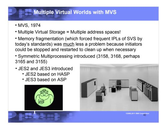
3032 processor shown without its PDU or CDU, with a 3851 MSS to the far left. 3505 reader and 3525 punch shown left of center, 3211 printer right of center. 3330 disk drives to the right rear. 3420 tape drives shown on the right.
