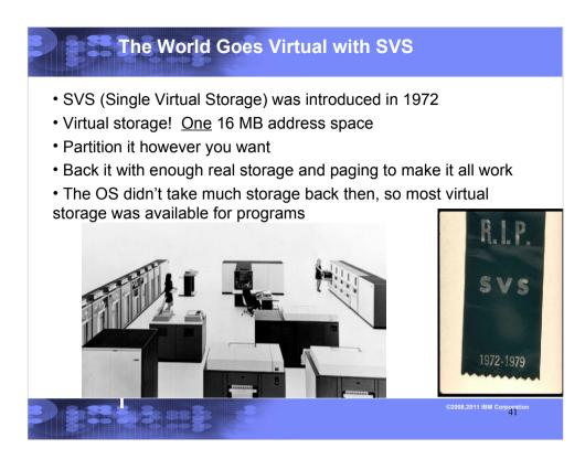
3155 processor shown, flanked by 3330 disk drives with a 3830 control unit on right, a remote 3215 console and 3420 tape drives on left, a rear view of two 1403-N1 printers in the right foreground with a 2821 control unit to their left. Behind the 2821 is a 2540 card reader/punch; to its right is a 3211 printer.
