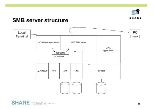
The SMB server runs as an authorized started task in its own address space. It accesses z/OS UNIX files on behalf of PC users. It can also access MVS data sets on behalf of PC users.
