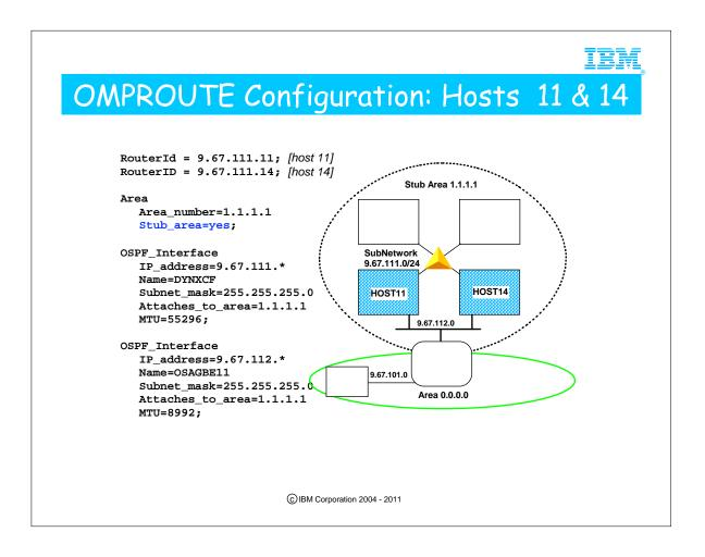
1. This configuration is identical to the first configuration for these two hosts except for the addition of Stub=yes on the area statement for 1.1.1.1
