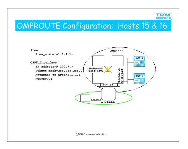
1. Like hosts 12 and 13 in the previous configuration, these hosts have a relatively simple configuration for attachment via Gigabit Ethernet to the OSPF network. Each may use a wildcarded definition.
