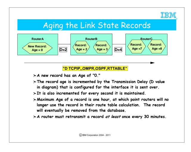
1. D TCPIP,,OMPR,RTTABLE displays the age of information about connections.
