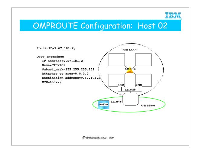
1. The main thing this configuration shows is that it is not necessary to define the backbone area (0.0.0.0) in routers that are in the backbone.
