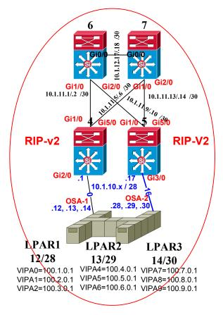
router-5#config-router router rip version 2 network 10.0.0.0
