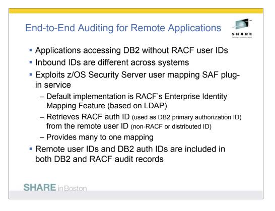
The default implementation of the z/OS Security Server RACF (SAF) user mapping plug-in makes use of EIM domain on z/OS. EIM is a LDAP server, which acts as a repository of mappings between an authenticated user registry name and a z/OS user ID.
