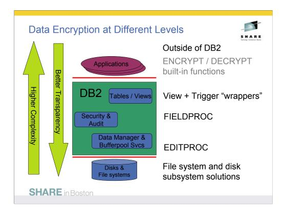
This diagram shows the range of places where data encryption can be performed. It is complementary to the prior page, which indicates some of the specific challenges.
