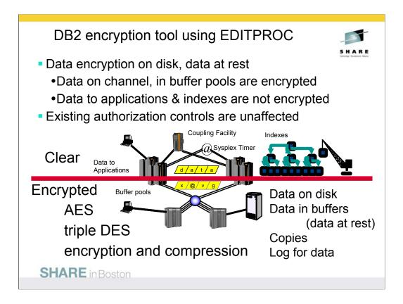
On this slide, data above the middle line is not encrypted and data below the line is encrypted.
