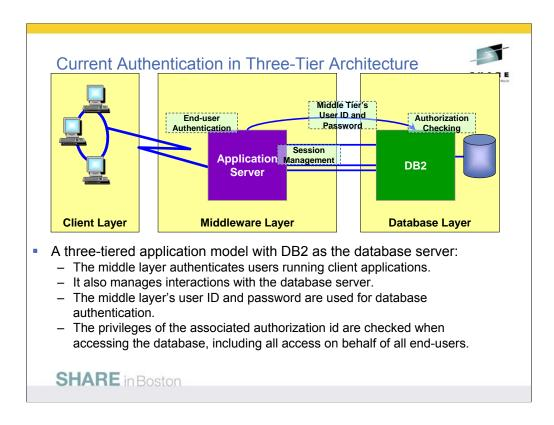
In a typical three-tiered application model with DB2 as the database server:
