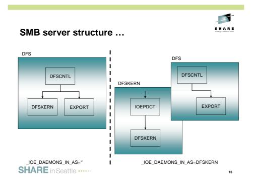
The DFSKERN process (which is the main server process) can run in the DFS address space (the default - shown on the left) or in its own address space (shown on the right). IBM recommends that you run DFSKERN in its own address space. This is accomplished by specifying \_IOE\_DAEMONS\_IN\_AS=DFSKERN in the /opt/dfslocal/home/dfscntl/envar environment variable. The DFSKERN JCL must also be available.
