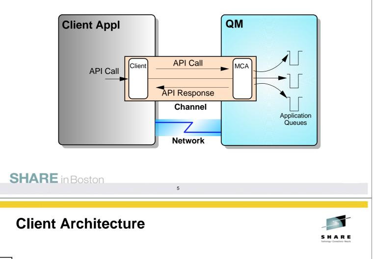
This diagram represents the WebSphere MQ client channel architecture. We are going to use this diagram throughout the presentation to illustrate the different client channel topics.
